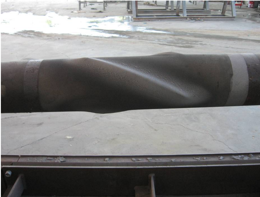
Figure 2: 8-11/16" Stabilizer on 7 5/8" Casing, as Sprayed
