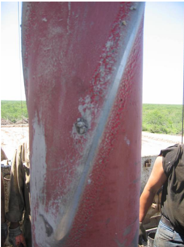
Figure 3: The same Stabilizer as in Figure 2 after Drilling over 2,000 feet
