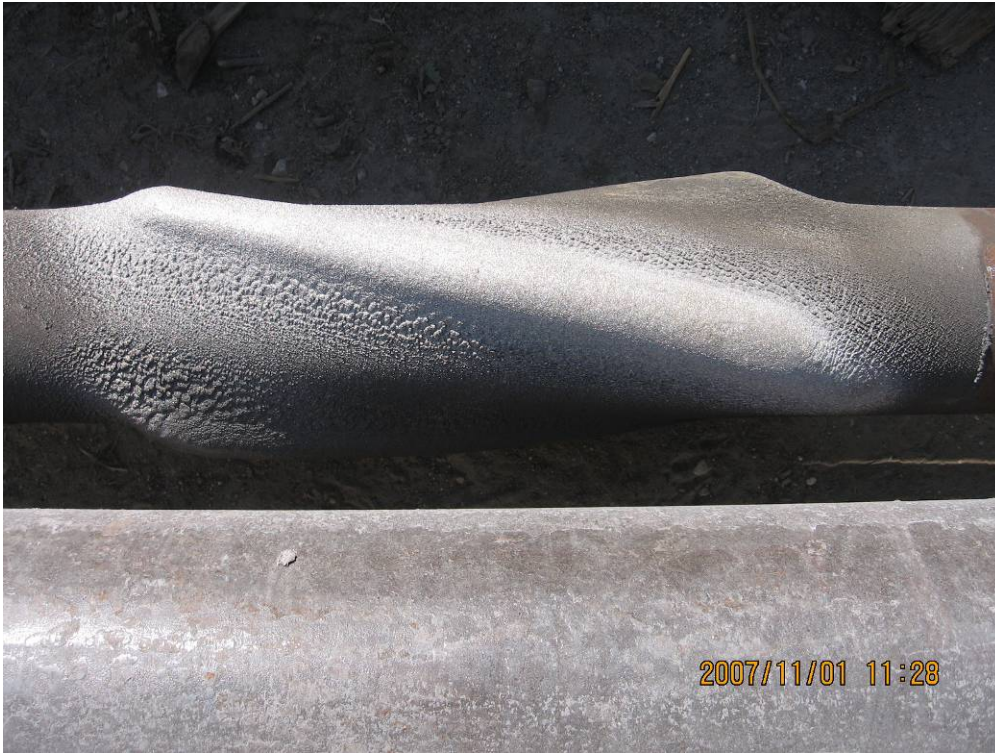
Figure 4: 6-3/16" Spiral Stabilizer on 4 1/2" Casing with 3/4" Gauge Blade Thickness
