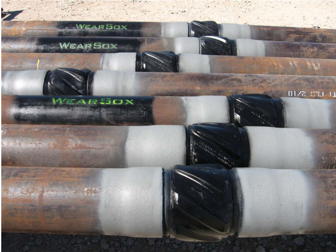
Figure 5: Typical Rotating Bowspring Centralizers with Internal Spray Metal Stops
