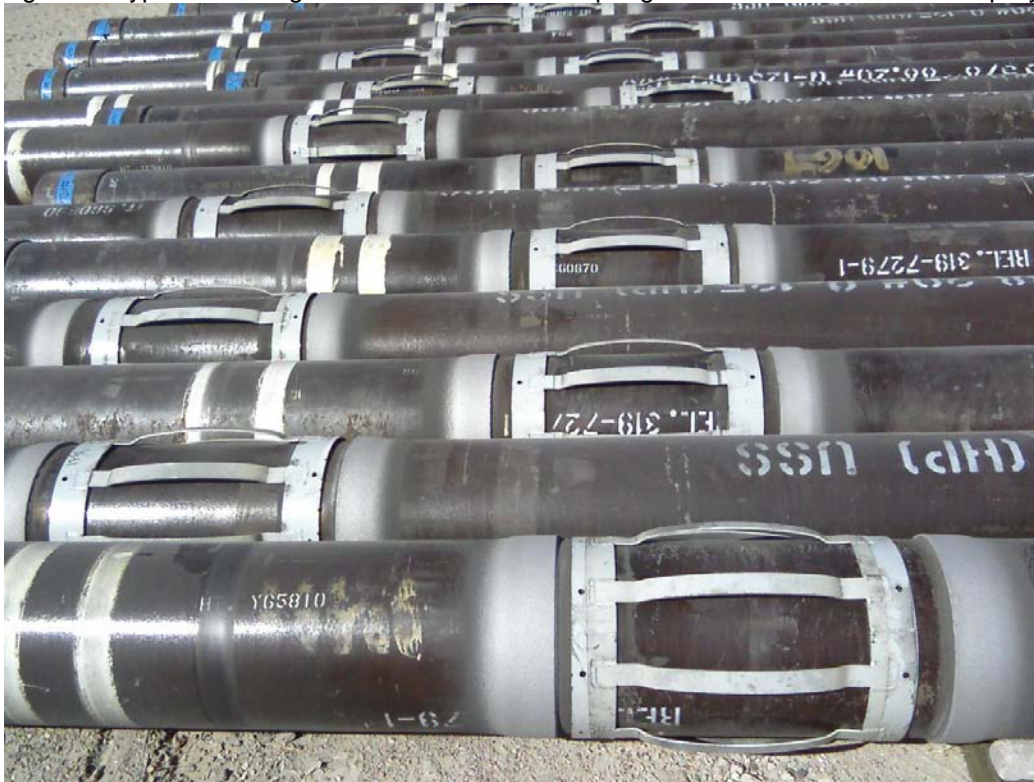
Figure 6: Typical Rotating “Close Tolerance” Bowspring Centralizers with External Spray Metal Stops
