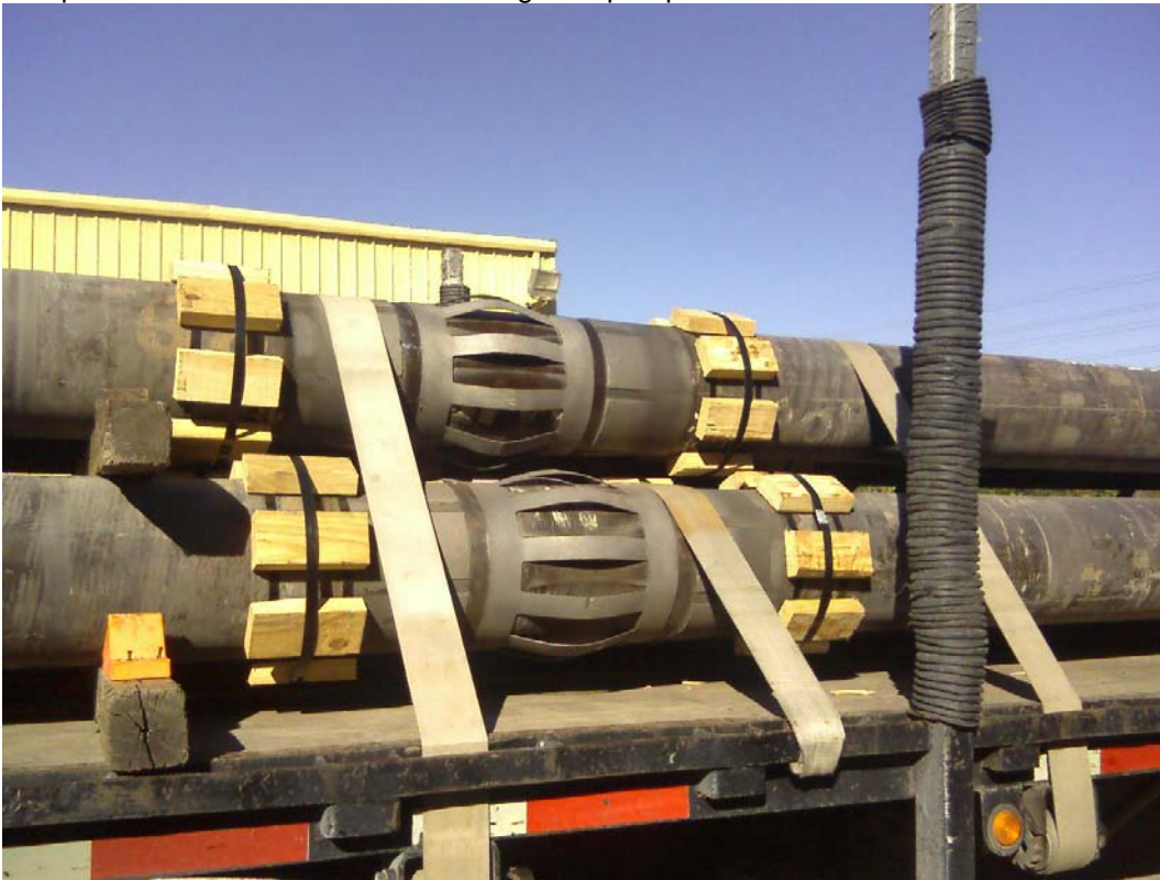
Figure 8: Typical Rotating “Very Close Tolerance” Bowspring Centralizers with External Spray Metal Stops, fluted to improve return mud flow. Also showing transport protection
