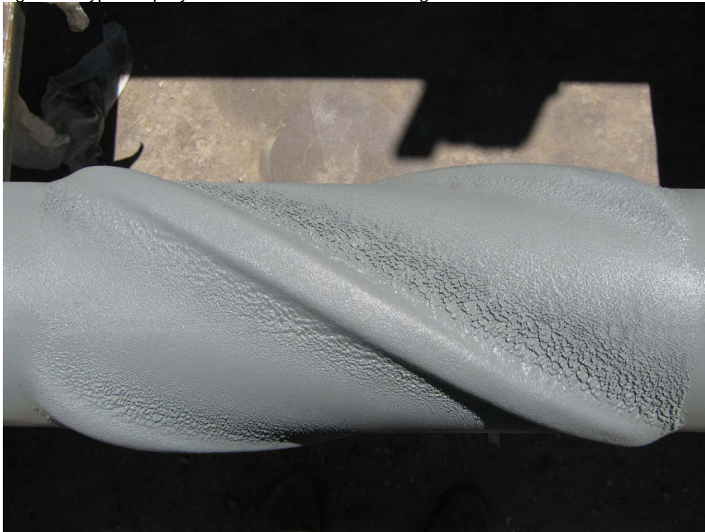
Figure 3: Typical Spray Metal 3-Blade Helical Casing Stabilizer
