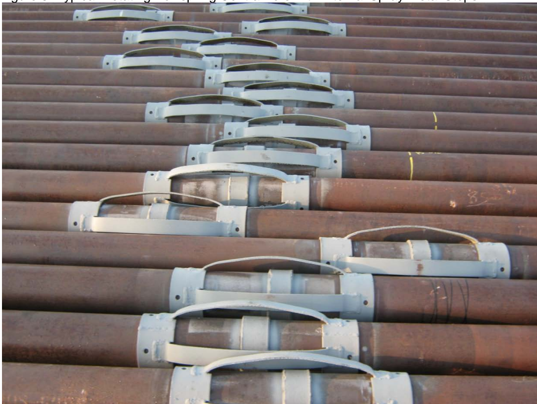
Figure 5: Typical Rotating Bowspring Centralizers with Internal Spray Metal Stops
