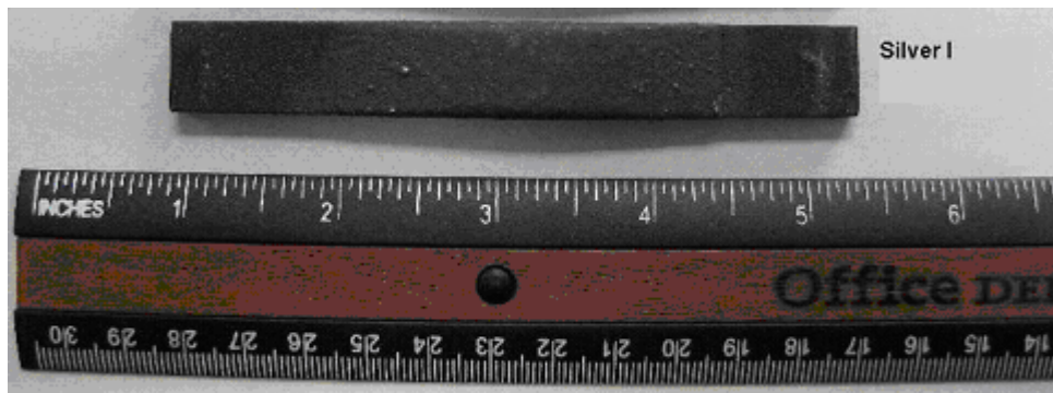
Figure 1. Thermal spray coating after autoclave SCC test
