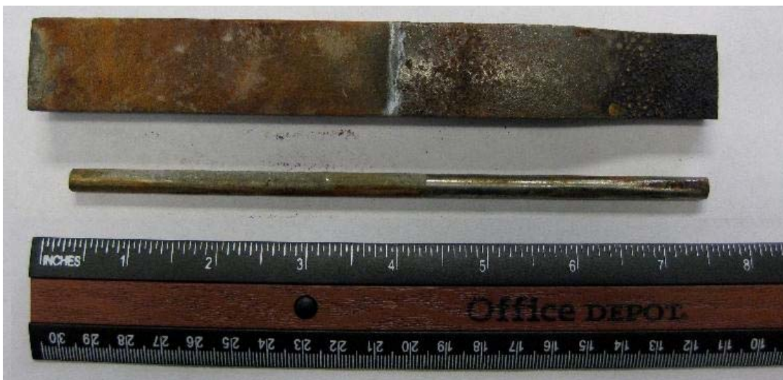
Figure 13. Synthetic seawater sample after 25 days in custom salt-spray test
