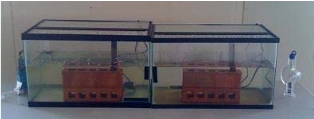
Figure 12. Photograph of custom-designed salt fog experimental arrangement
