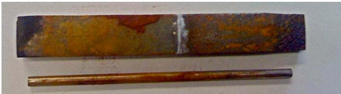
Figure 15. Natural seawater sample after 25 days in custom salt-spray test
