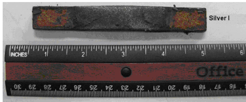
Figure 3. Thermal spray coatings after 312-hour salt spray (fog) test
