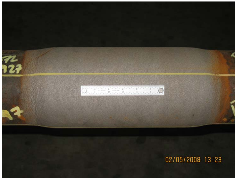
Figure 4 Center WearSox band did not develop any cracks.
