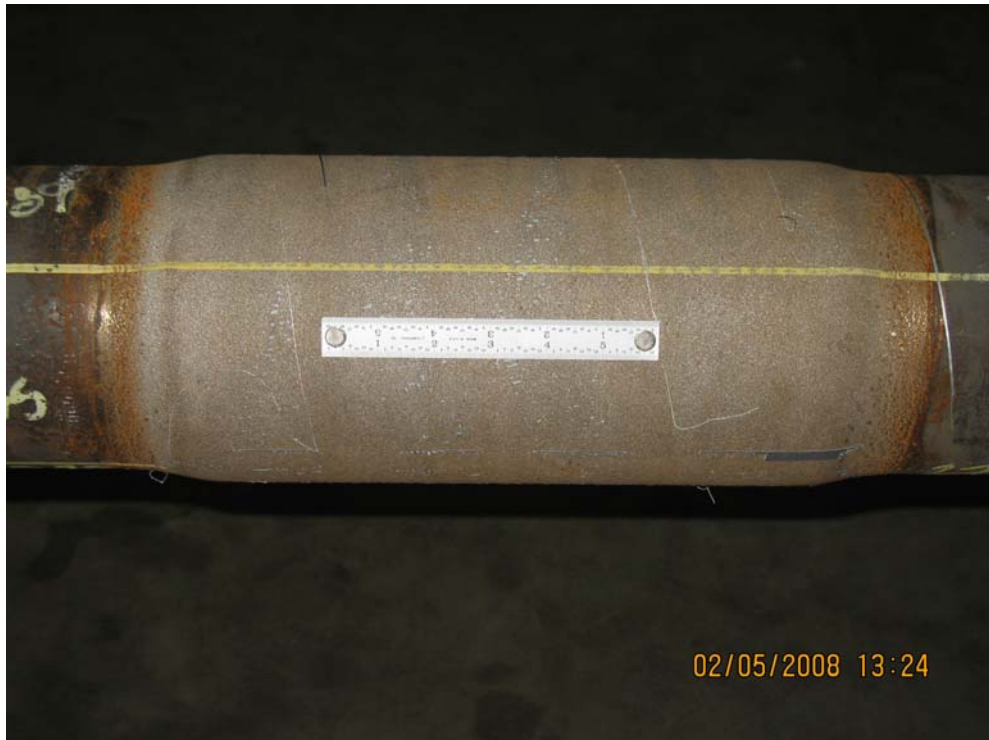
Figure 5 WearSox band on "dead" end that did not crack.
